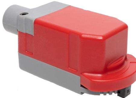
Siral offers three zone series non-fail safe actuators. An On/Off, floating 24V version, a On/Off, floating (100 - 250V) version and a Modulating ((0)2 - 10V) 24V version. All actuators mount directly to all the Siral zone ball valves.
