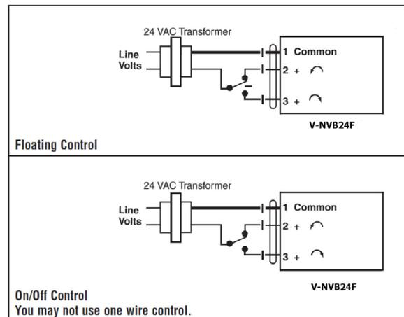
Direct/Reverse acting switch is under wiring cover.
